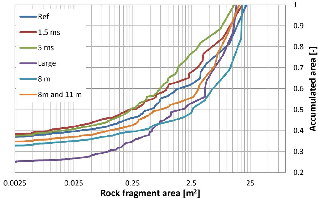
Figure 8. Accumulated area plot for vertical cut V4 (at the symmetry line) for all simulated cases.
