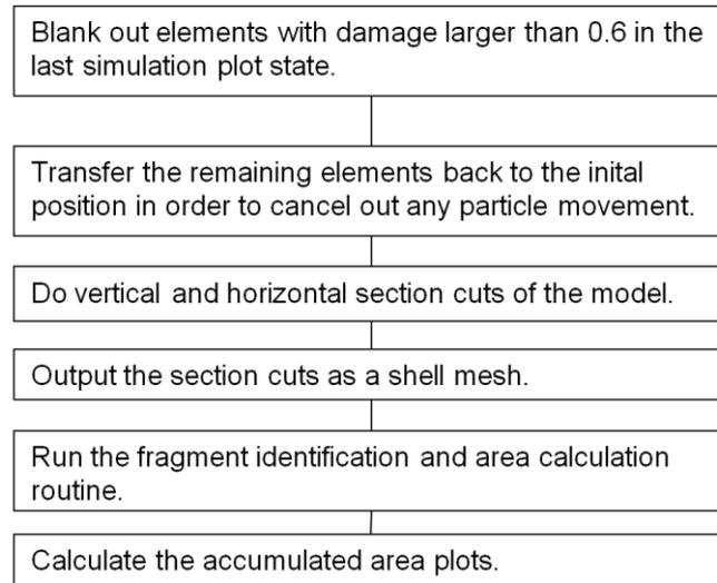
Figure 3. Procedure for fragment size calculation.
