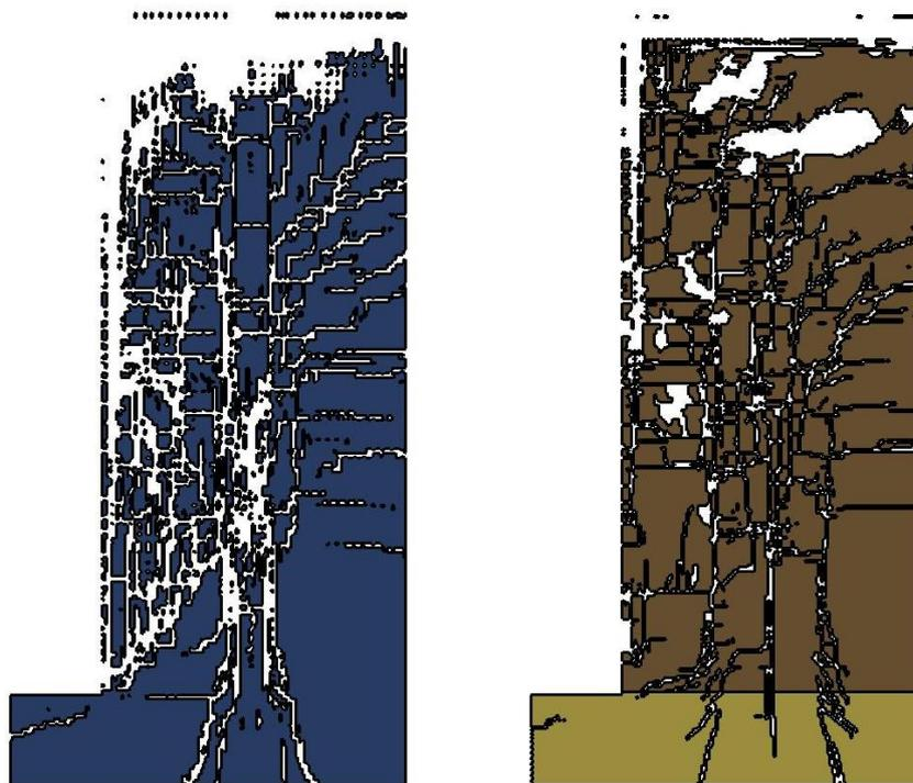
Figure 9. Fragmentation pattern for vertical cut V4 (see Figure 4 for location of evaluation cuts) and Case 1: 8.7 m hole spacing (left) and Case 4: 12.3 m hole spacing (right). White areas are considered to be fully crushed (damage level > 60 % and thus a fragment size less than 50 x 50 mm).
