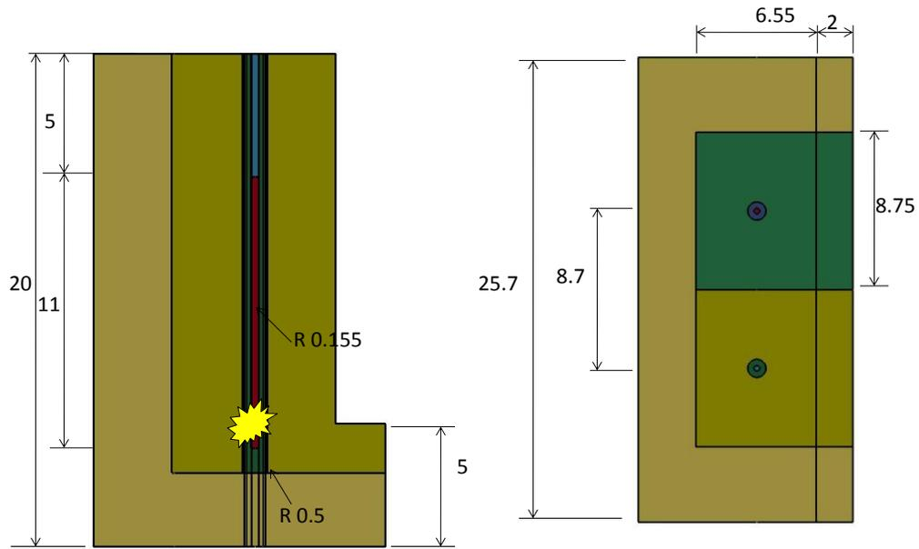
Figure 1. Geometry of the finite element model of two blast holes: vertical cross-section(left) and horizontal plan view (right).
